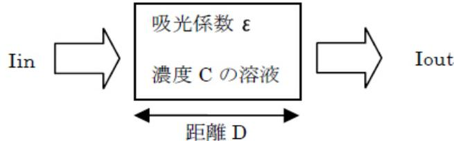
$$-\text{Log}(I_{out}/I_{in}) = \text{溶液の吸光係数} (\epsilon) \times \text{溶液の濃度} (C) \times \text{距離} (D)$$
